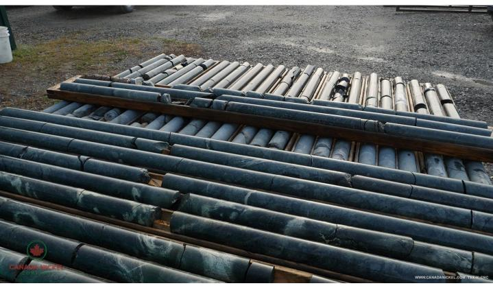
Core Samples collected during Canada Nickel's extensive, ongoing exploration of Crawford and its neighboring deposits.
