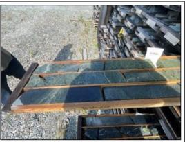
(B) Drill core from diamond drill hole DEL22-01; NQ core with a diameter of 47.6 millimetres (Siriunas, 2024).
