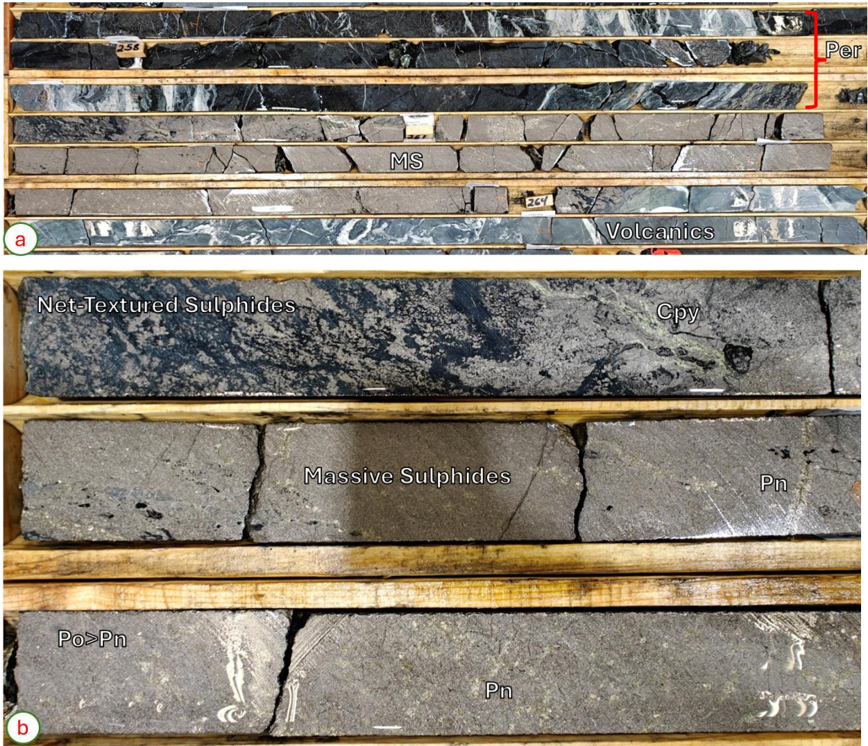
Figure 2 – BAN24-18, core pictures a (256.1-267 metres) ,b (260.3-263.4 metres),c (select intervals 257.2-262.7 metres )
