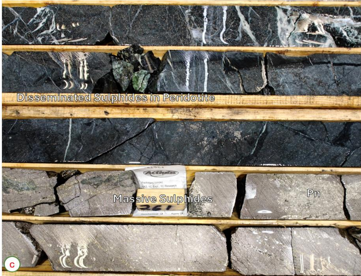
a) Peridotite to Massive sulphide, to volcanics; b) Net-texture sulphides (Po (Pyrrhotite)>Pn (Pentlandite)>>Cpy (Chalcopyrite); c) Disseminated sulphides on peridotite, into massive sulphides Po>Pn;
