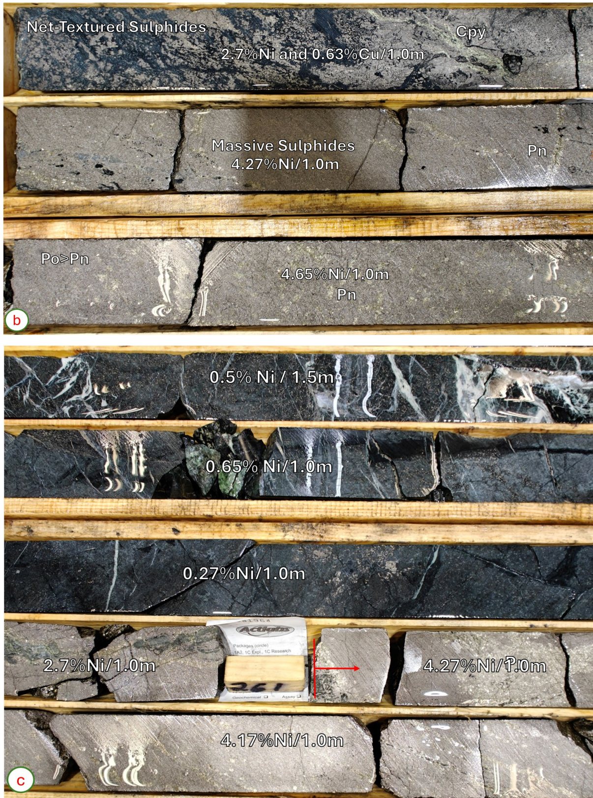
a) Peridotite to Massive sulphide, to volcanics; b) Net-texture sulphides (Po (Pyrrhotite)>Pn (Pentlandite)>>Cpy (Chalcopyrite); c) Disseminated sulphides on peridotite, into massive sulphides Po>Pn;
